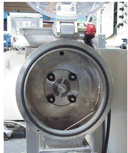
Single Screw Duplex Vacuum Plodder
